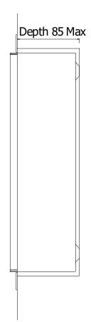
The front of the Master Station should protrude by 10mm to allow the doors to open fully in operation.
